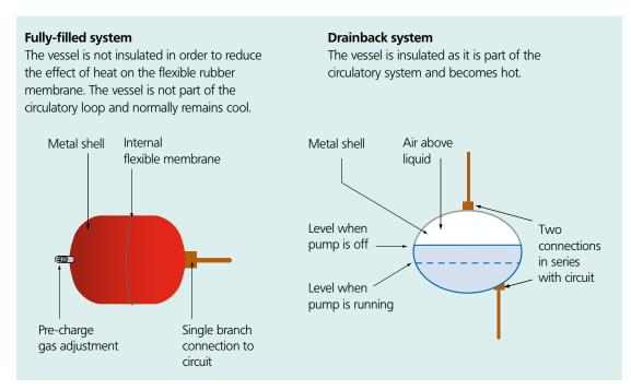
Figure 6 Schematics of two types of vessel used in SDHW
