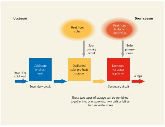
Figure 2 The movement of heat and fluid through a SDHW system
