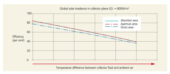
Figure 5 Simplified efficiency graph to EN 12975
