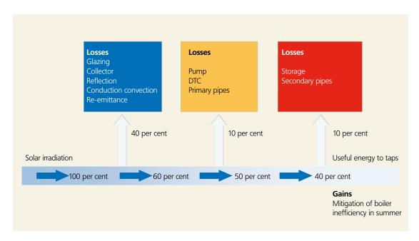
Figure 10 Schematic showing losses from SDHW systems
