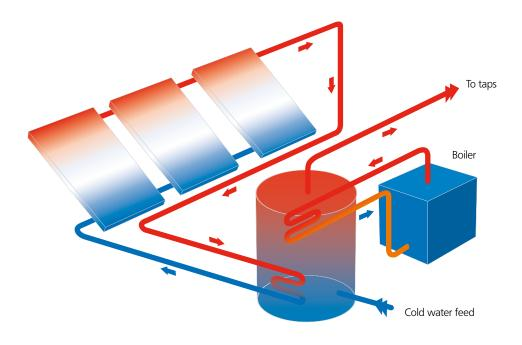
Figure 1 Solar domestic hot water heating schematic
